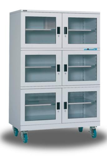
SDC-1206-01 is equipped with HEPA filter and dry unit, controlling cleanliness and humidity simultaneously. Air cleanliness class 100, humidity 1%RH. It is designed for moisture sensitive SMD packages to comply with IPC/JEDEC J-STD-033C, most suitable for clean room use. Two powerful dry units installed, making it very suitable for operation with frequent approach.
