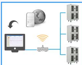
❖ Network system for humidity and temperature (including module and software)
